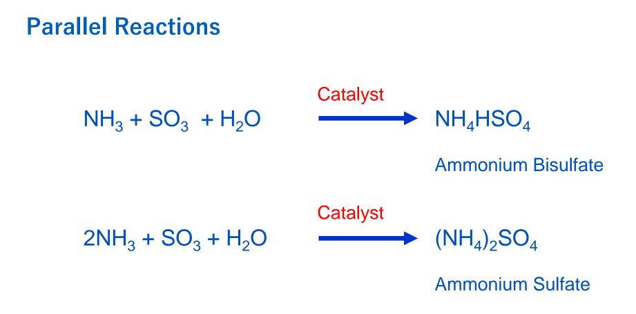
Both salts form at flue gas temperatures below 320°C
